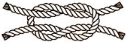
Square Knot – Attach two ropes of the same size
