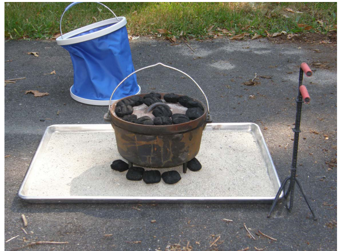
Dutch oven on a fire pan. Pan has an insulating layer of sand. Optional: can support pan on bricks. (A lid lifter is on the right.)
